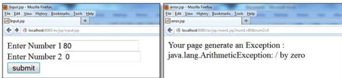
Figure 7: Exception handling at application level by using deployment descriptor
